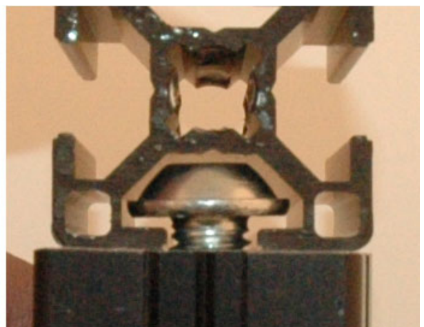
Safety screw not touching top (correct)
